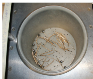
Picture II: Testing machine used at John Innes Centre to determine pod strength for five commercial OSR varieties.
